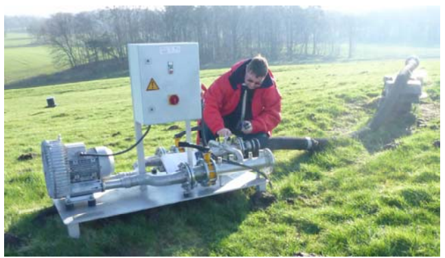
Illustrations 3, Employment of the mobile DMF V small-scale flare with a mobile gas analysis and flow measurement at the Vechta - Tonnenmoor [DAS - IB GmbH] site as a substitute for the initial gas disposal in the brickworks, and a theoretical and practical air injection (picture on the top right and below)
